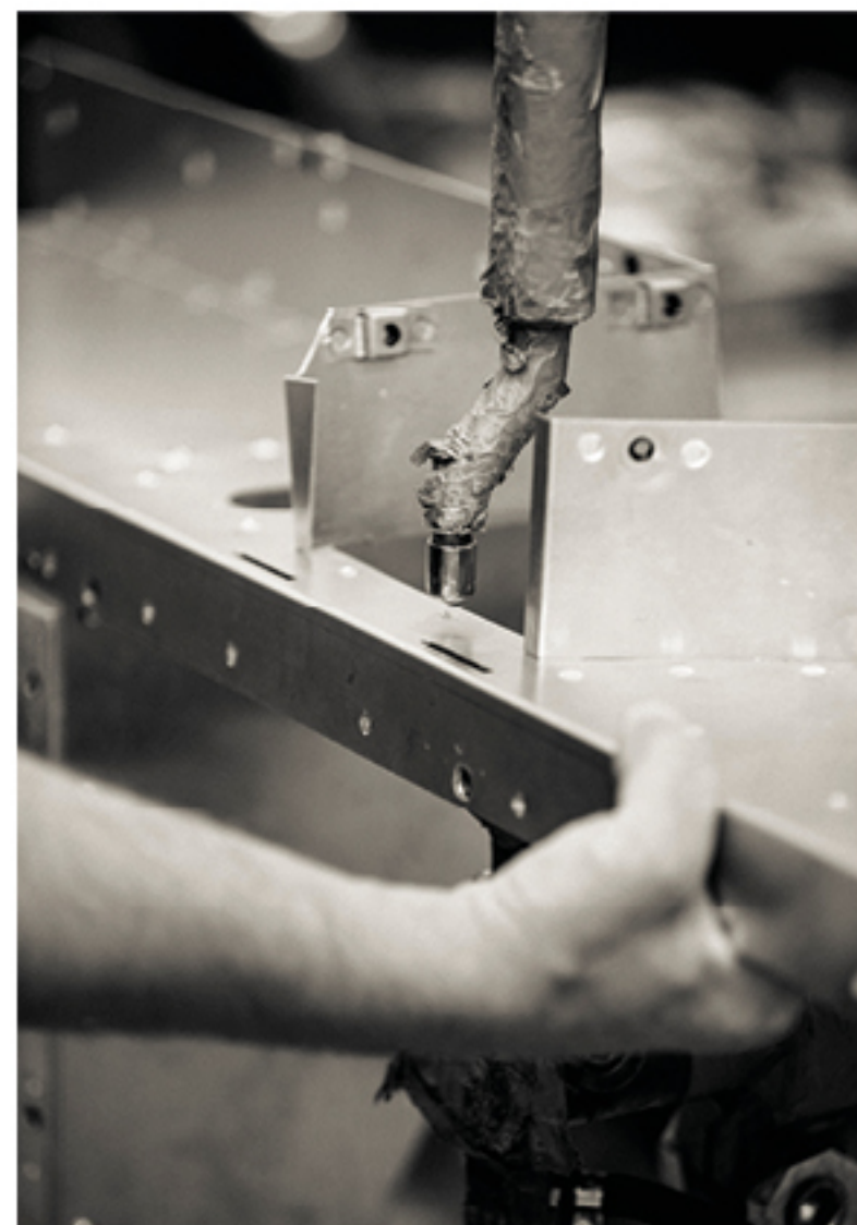
Spot welding a post-1500 seat box together on CKD's custom-made 150kva spot-welder
